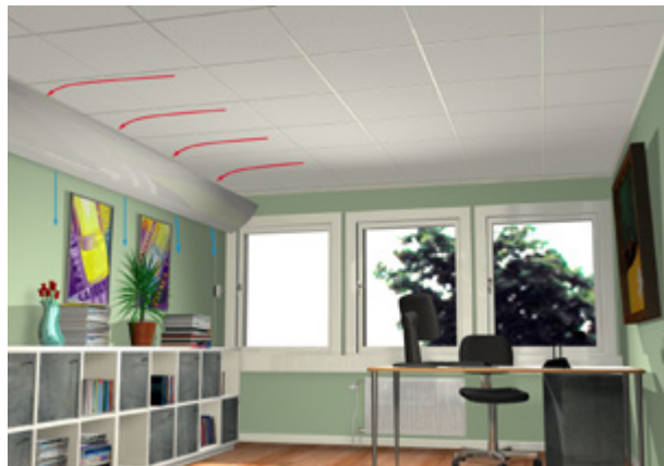
Picture 4. Plafond D with air injection across the wall.
