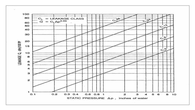
Prior to the 2013 version ASHRAE Standard 90.1 required Leakage Class 6 for rectangular metal and round flexible duct and Leakage Class 3 for round and flat oval metal duct.
