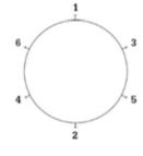
Always start the first fastener at the largest radial gap between fitting and duct. Be sure to achieve even distribution around the circumference.
