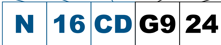
= 16" Diameter Coupling Duct In Galvanized 24 Gauge
