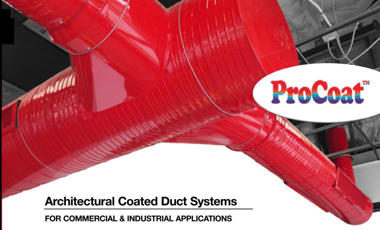
ProCoat<sup>™</sup> is a "baked on" powder coated system applied to the outer shell of the HVAC air duct system. The primer coat is a zinc-rich epoxy. It provides superior chemical resistance -- equal to, or better than PVC. The polyester top coat protects the base coat and adds a clean glossy finish.
