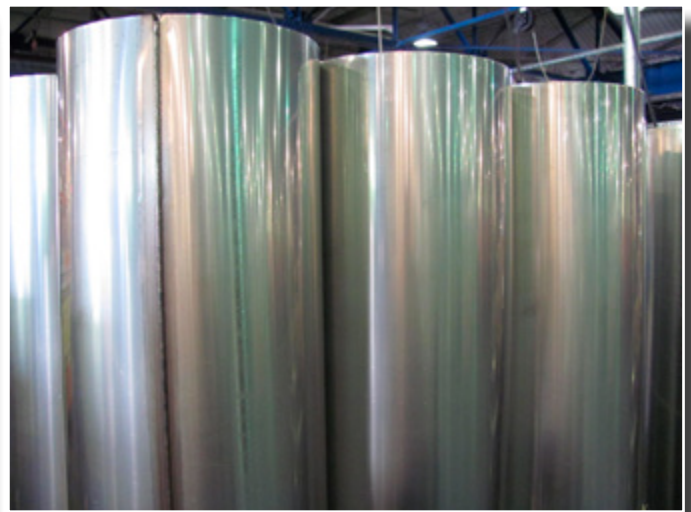
longitudinal-seam welded duct
